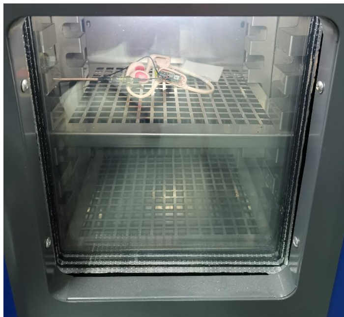
Photograph 2: Set-up for Radio Spectrum Testing, Extreme Condition
